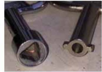
Common keys required for opening cabinets
