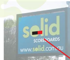
If you have a faulty row of modules replace the right (red) module first. This faulty module is likely to be sending bad data to the row.
